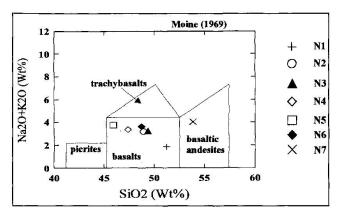
Fig. 7 The samples except N7 show a basaltic composition; N7 is basaltic andesitic.
