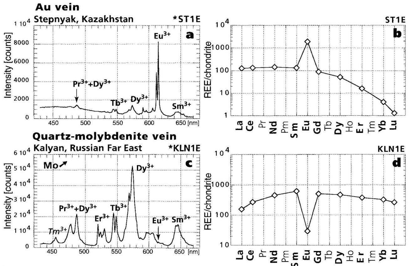
Fig. 2 Comparison of XLT spectra and chondrite-normalised REE data obtained by isotope dilution data. The Stepnyak Caledonian gold and scheelite-bearing quartz-carbonate-sulphide veins are situated inside a granodiorite stock and the intruded, altered volcanic-sedimentary rocks. The Mesozoic molybdenite-scheelite quartz veins ( $\pm$  fluorite, minor arsenopyrite and pyrrhotite) at Kalyan are situated in altered volcano-sedimentary rocks.
