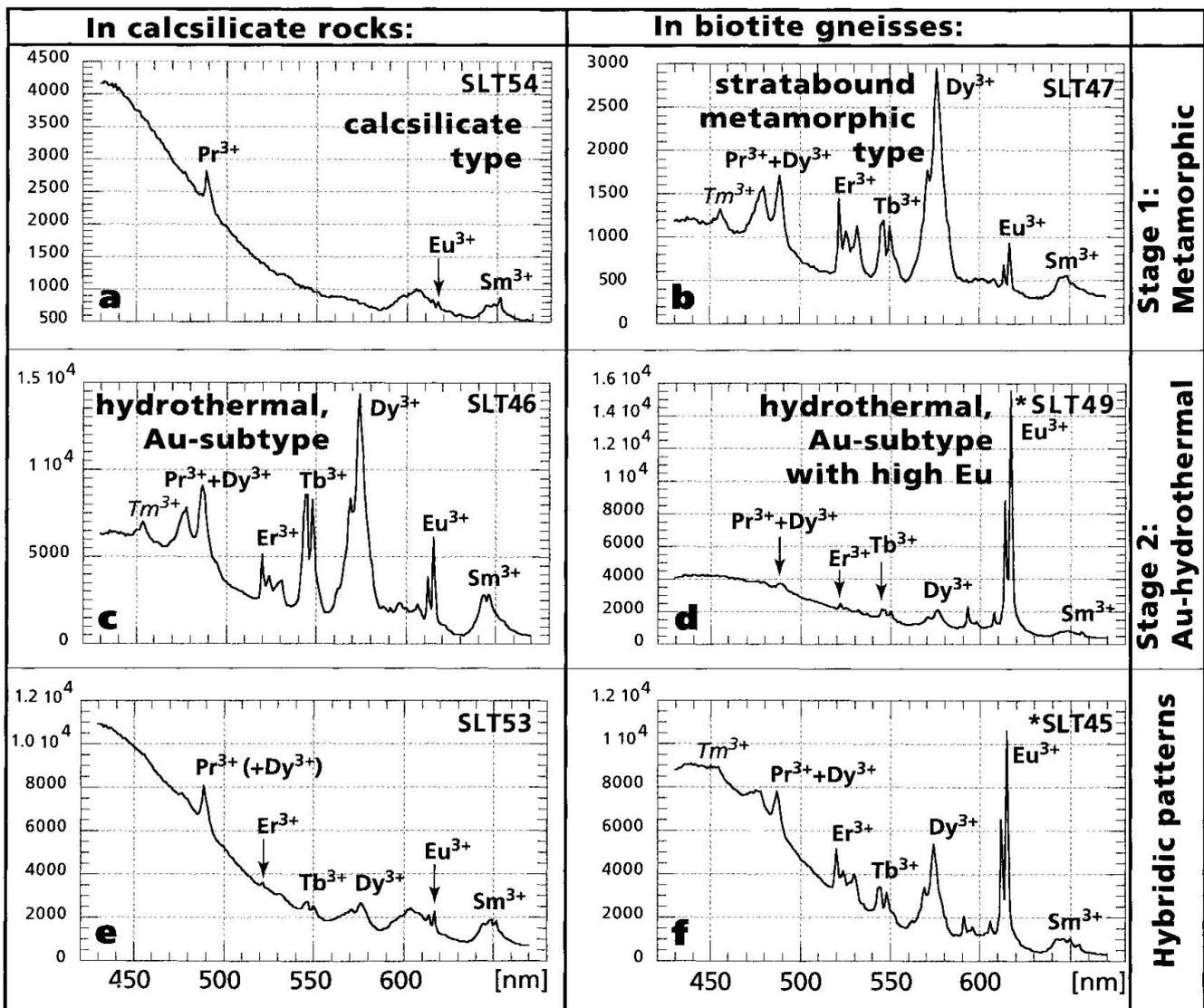
Fig. 9 Different types of XLT spectra of scheelites from Sotto Ceneri (Switzerland and Italy). Vertical axes are intensities [counts]. The complexity of the spectra collected in these scheelites may be explained by hydrothermal remobilisation of a stratabound scheelite mineralisation.
