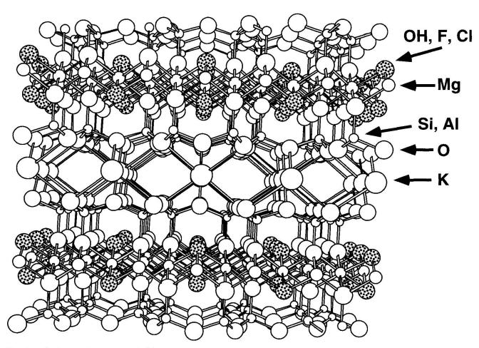
Fig. 1 Ideal crystal structure of phlogopite as shown in perspective along the a axis.
