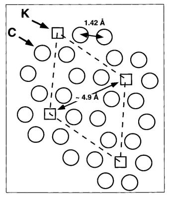
Fig. 5 Mineralogical relationship between the (001) mica surface and the (001) in graphite The unit cell for K sorbed on graphite (indicated in the figure) was experimentally determined by BENNICH (1996).
