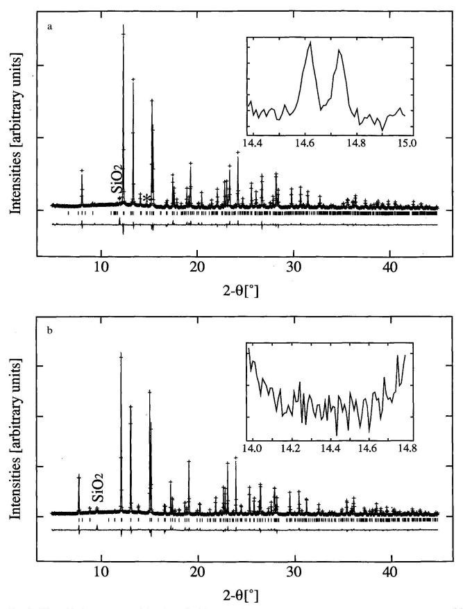
Fig. 1 Rietveld plots of Mal00 (a) and Mal10 (b), respectively. The peaks labeled with  $SiO_2$  are due to quartz (a) and cristobalite (b) respectively. The insets show an enlargement of the area where the strongest non-overlapping  $P2_1/a$  specific peaks (22 $\overline{1}$  and 21 $\overline{2}$ ) are expected. These two peaks are also marked with a star in figure 1a. Their absence in figure 1b indicates space-group A2/a. These peaks were observed only in Mal00.
