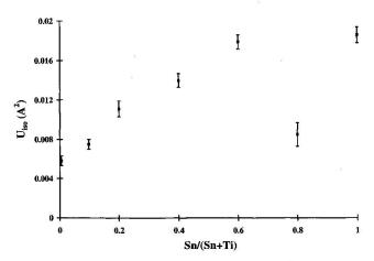
Fig. 7 Isotropic displacement parameters ( $Å^2$ ) of Ca as a function of Sn-content. The increasing trend for higher Sn-contents and thus Ca-polyhedral volume is interpreted as a manifestation of a flatter potential well due to the sterically caused stretching of the Ca-site.
