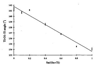
Fig. 5 Pivot-angle (Ti-O1-Ti) of the octahedral chains as a function of Sn-content. The decreasing trend reflects steric strain within the structure. This effect is partly compensating for the octahedral volume increase which is in competition to the geometric requirements of the Ca-chains. The line serves as a guide to the eye.
