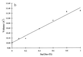
Fig. 3 Volumes as a function of Sn-content. Polyhedral volumes were calculated with the program "volcal" by L. Finger and Y. Ohashi (http://www.lmcp.jussieu.fr/sincris/logiciel/prg-volcal.html). Solid lines represent linear regression fits through data.
