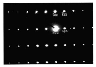
Fig. 2 Selected-area electron diffraction (SAED) pattern of a Mal10 crystal. Note the absence of the k + l = odd reflections (such as 112) indicating space group A2/a.
