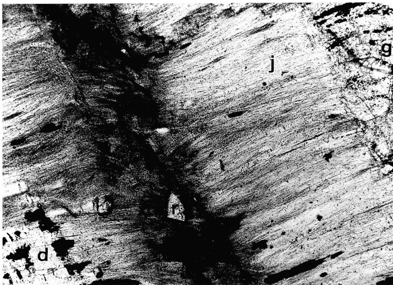
Fig. 1 Microphotograph of a johninnesite veinlet. j = johninnesite, r = roméite, d = dolomite (belongs to the veinlet), g = embedding ore, consisting mostly of dolomite, hematite, jacobsite, and manganian muscovite. Transmitted light, field of view 1.25 \times 0.92 mm.
