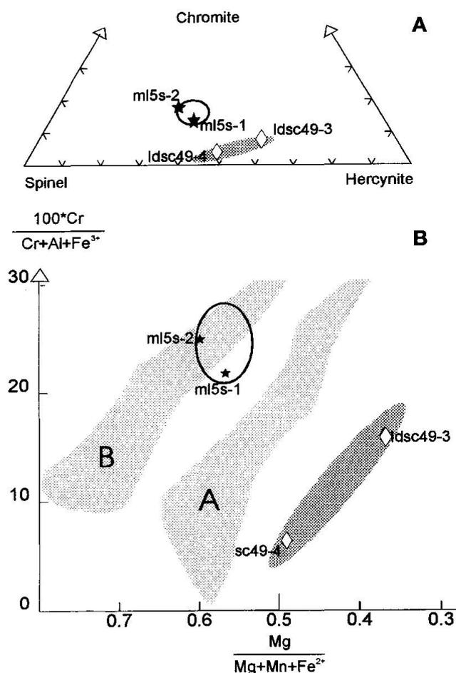
Fig. 6 (A) Classificatory diagram of spinel in ultramafic rocks. (B) Composition of spinel in terms of  $\text{Mg}/(\text{Mg} + \text{Fe}^{2+} + \text{Mn})$ , and  $\text{Cr}/(\text{Cr} + \text{Al} + \text{Fe}^{3+})$ : Solid line: field of peridotite, dark shade area: pyroxenite; full star = peridotite; diamond = pyroxenite. Light shaded fields represent spinels in cumulitic peridotites (A) and mantle peridotites (B) from Balmuccia (Ivrea Verbano Zone, GARUTI et al., 1980, Fig. 6).
