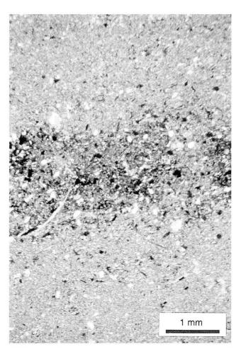
Fig. 2 Crossed polars microphotograph of the LST ash level (darker in color) interbedded within lacustrine marls.
