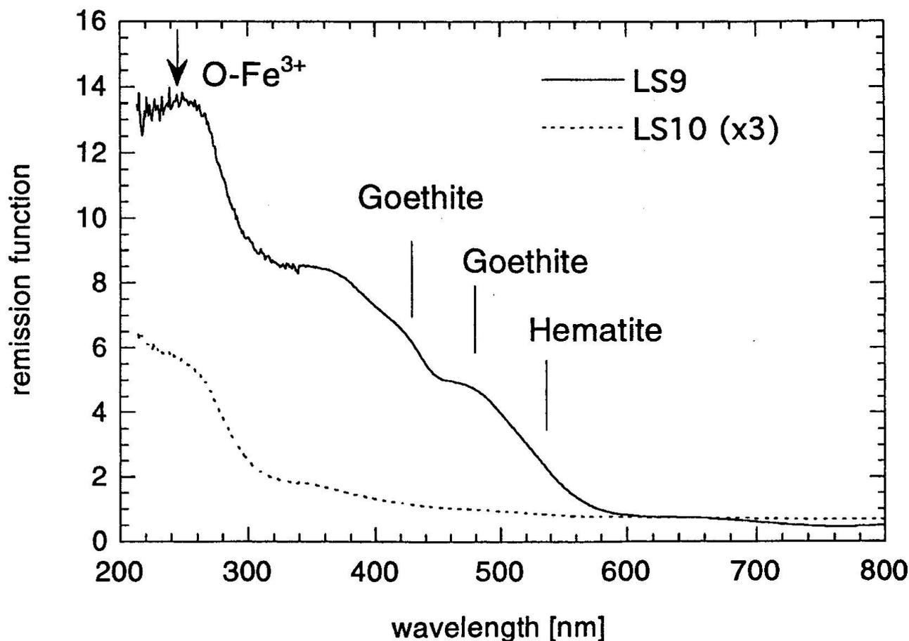
Fig. 5 Diffuse reflectance spectra of LS5 and LS10 samples in the UV-visible range. Arrows indicate the positions of absorption bands assigned to  $\text{Fe}^{3+}\text{-O}$  charge transfer and to the various Fe-oxides. Spectrum of sample LS10 is increased by a factor of three.
