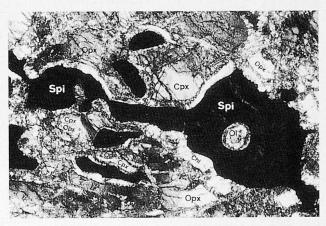
Fig. 3 Photomicrograph of a typical elongated spinelpyroxene cluster texture. Crossed polarizers. Long dimension of the photo is 3.5 mm. The interior of the cluster is essentially made of pyroxene and spinel, olivine is absent. Note that spinel is bordered by chlorite which grew during retrograde amphibolite-facies metamorphism. Abbreviations are Ol, olivine; Opx, orthopyroxene; Cpx, clinopyroxene; Spi, spinel; Chl, chlorite.
