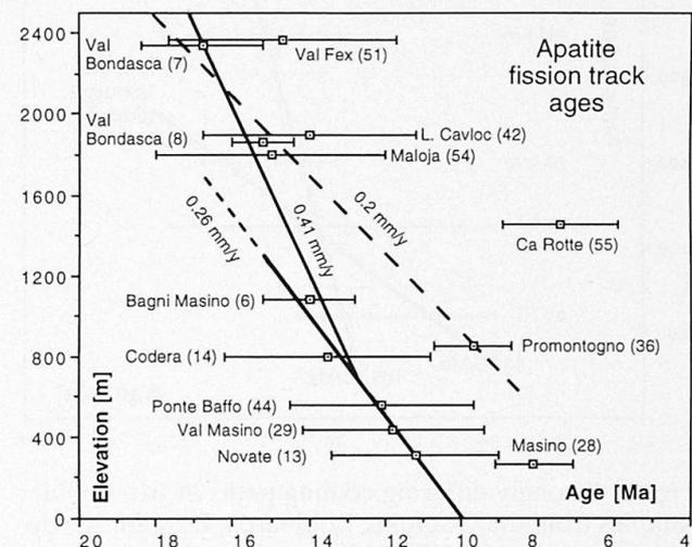
Fig. 8 Elevation versus age diagram of apatite fission track data from WAGNER et al. (1979). Error bars represent 2  $\sigma$  errors. The samples are labeled by the sampling locality and a location number referring to figure 2. An alternative hypothesis for the northern MB area (dashed line) yields an exhumation rate of 0.2 mm/year which is very similar to the exhumation rate of 0.26 mm/year obtained for the Val Masino and Novate areas.
