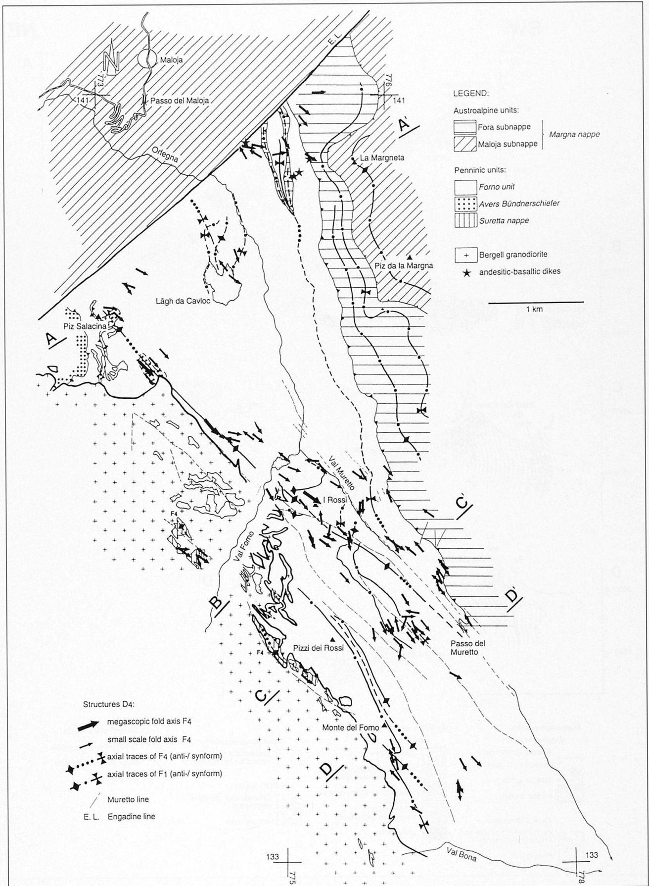
Fig. 7 Map of deformation phase D<sub>4</sub> including fold axes and axial traces.
