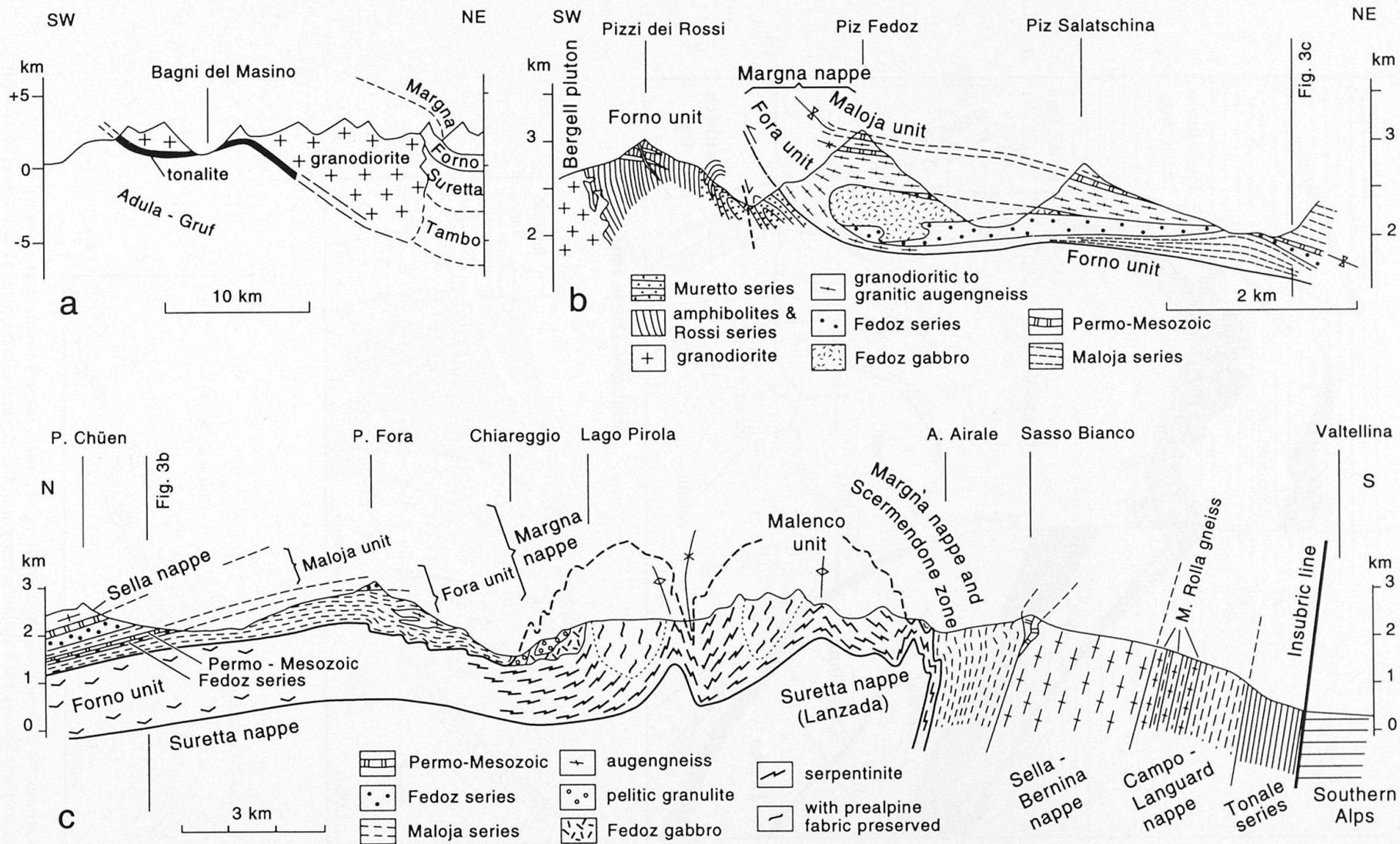
Fig. 3 (a) Synthetic SW-NE section through the Bergell pluton, after BERGER and GIERÉ (1995).
