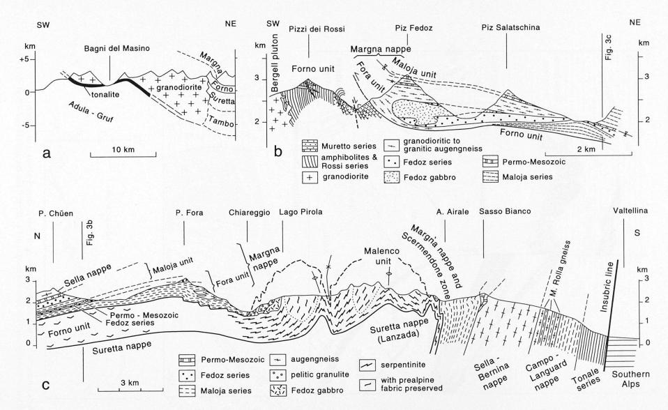
Fig. 3 (a) Synthetic SW–NE section through the Bergell pluton, after BERGER and GIERÉ (1995). (b) Detailed SW–NE section through the eastern margin of the Bergell pluton, after Spillmann (1993).
