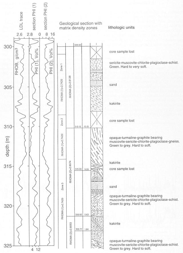
Fig. 3 Small scale correlation between RHOB, PHI (1), PHI (2) and the geological section. The accuracy of the depth position of core samples decreases with increasing depth, therefore correlations must be done with much care, and by consulting other log traces (e.g. FMS-image).
