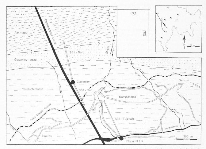
Fig. 1 Simplified map with the locations and traces of the three NEAT boreholes. This work only deals with SB3-Tujetsch. Bold line = trace of the planned Gotthard base tunnel. Inset: A = Andermatt, B = Biasca, C = Chur, D = Disentis, G = Glarus, I = Ilanz, L = Locarno, S = Sedrun, T = Thusis. Coordinates correspond to the 1 km grid of the "Schweizerische Landeskarte 1:25'000".
