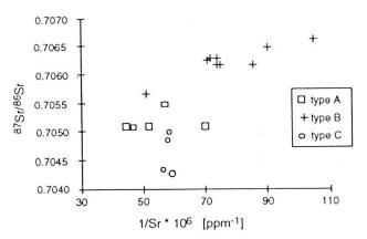
Fig. 2  $^{87}$ Sr/ $^{86}$ Sr vs 1/Sr of barites from the different types of ore occurrences.
