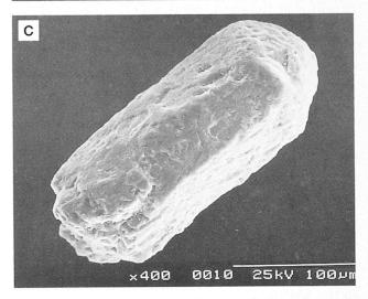
Fig. 4 REM-pictures of apatite crystals from the unaltered trachyte (A), the propylitically altered porphyritic syenite (B) from Skouries, and from the phyllically altered diorite porphyry at Fisoka (C). Skale bars correspond to  $100~\mu m$ . Corrosive effects can only be observed in (C), whereas apatite in the other two cases preserved its shape under conditions prevailing during post-magmatic alteration.
