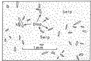
Fig. 4 Reproduced from coloured photomicrographs. (a) Crystallographically oriented lamellae of diopside in a grain of bastite. (b) Serpentine matrix containing very fine grained, prismatic crystals of diopside.
