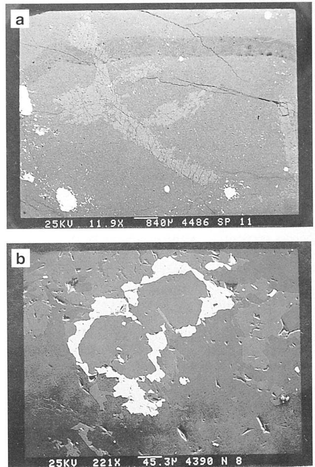
Fig. 3 SEM images (scaled in  $\mu\text{m}$ ). a) Elongated grains of olivine (light grey) in a serpentine matrix (darker background). b) A rim of magnetite (bright white) around olivine (middle of the picture) in a serpentine matrix (black background).
