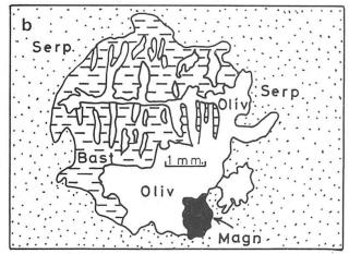
Fig. 2 Reproduced from coloured photomicrographs. (a) Thin veins of olivine traversing a grain of bastite. (b) Development of olivine at the expense of bastite.
