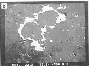
Fig. 3 SEM images (scaled in  $\mu$ m). a) Elongated grains of olivine (light grey) in a serpentine matrix (darker background). b) A rim of magnetite (bright white) around olivine (middle of the picture) in a serpentine matrix (black background).
