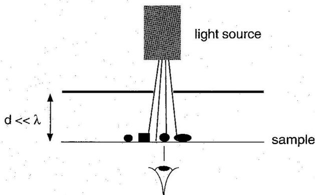
Fig. 1 Generic scanning near-field optical microscope (SNOM) setup: a subwavelength light source is raster-scanned across the sample at small distance.
