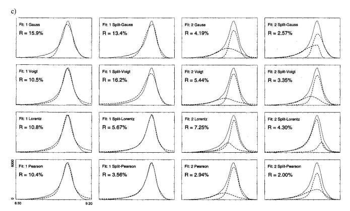
phase), but probably by the impact of grinding on the edges of mica flakes. c) Such an asymmetric reflection cannot be fitted with one single mathematical function, but with a Split-Pearson curve, STERN et al., 1993.
