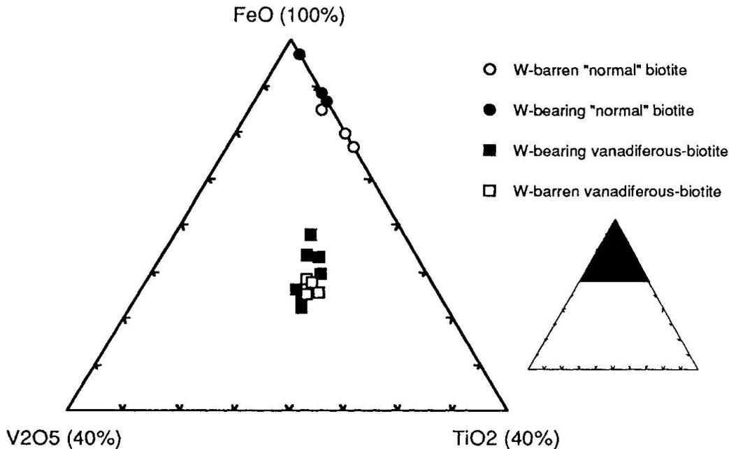
Fig. 7 FeO-V<sub>2</sub>O<sub>5</sub>-TiO<sub>2</sub> ternary diagram for W-bearing and W-barren biotites in samples of the paragneiss series. W-bearing biotites are Fe-richer than W-barren ones both in the graphitic schists (vanadiferous-biotites) and in the metagreywackes ("normal" biotites).
