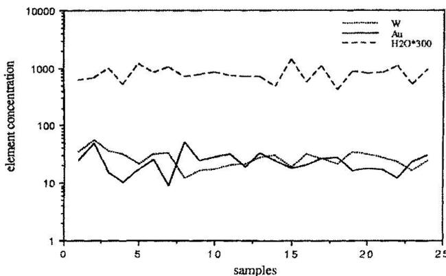
Fig. 6 Variation in the concentration of Au and W in comparison to that of H<sub>2</sub>O, in samples from the paragneiss unit. Au and W do not display a good correlation with water content of the rock.
