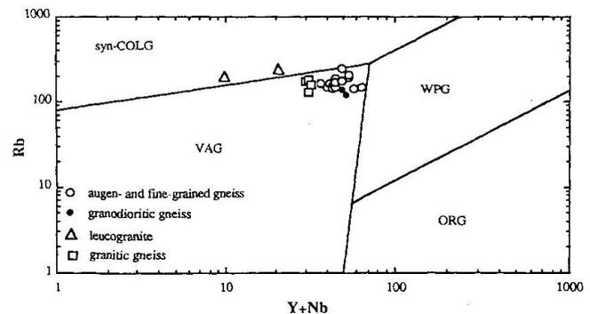
Fig. 3 Diagram showing a volcanic arc environment for the emplacement of the orthometamorphites and a syn-collisional environment for the leucogranite (from PEARCE et al., 1984).
