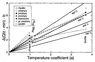
Fig. 4 Isotherm plot (Javoy et al., 1971) for mineral separate data from the Vallorcine granite. The temperature coefficient a is related to  $\Delta$  (Qtz-min) – b by equation 1. Temperature coefficient data are taken from Javoy (1977) assuming an  $X_{\text{anorthite}}$  component in plagioclase of 0.2. Shown are isotherms for 400 °C, 500 °C, 600 °C and 700 °C.
