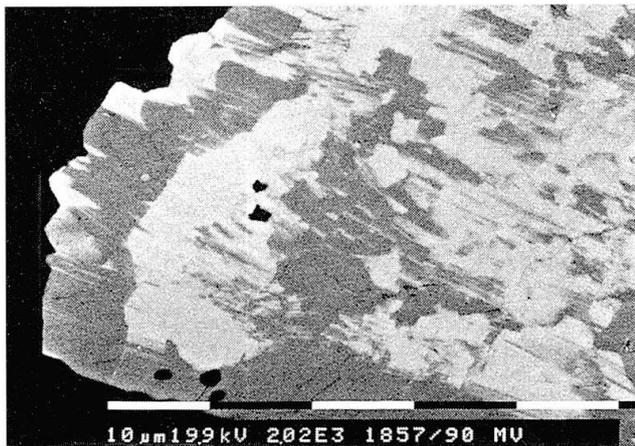
Fig. 5 Back-scattered electron image of orthopyroxene (En<sub>50</sub>Fs<sub>50</sub>; in white) and diopside (dark gray) intergrowth. Quartz is black (sample Vn3).
