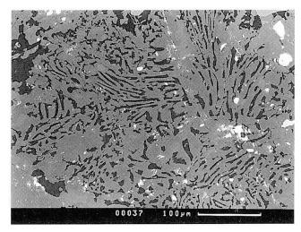
Fig. 4 Back-scattered electron (BSE) image of sodic diopside (up to 15 mole % of Jd; pale gray) and oligoclase (Ab<sub>90</sub>An<sub>10</sub>-Ab<sub>80</sub>An<sub>20</sub>; black) symplectite after omphacite (sample Ua36, Unteralptal).
