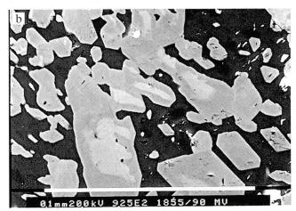
Fig. 6 a: Amphibole (Mg-hornblende and edenitic hornblende; gray) albite (black) intergrowth. b: Amphibole (Mg-hornblende and edenitic hornblende; gray) albite (black) intergrowth replacing diopside (pale gray cores in the Am) and oligoclase (not visible) symplectite after omphacite (BSE image; sample Vn10 from Alpe Toma, Val Nalps).
