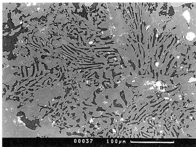
Fig. 4 Back-scattered electron (BSE) image of sodic diopside (up to 15 mole % of Jd; pale gray) and oligoclase ( $\text{Ab}_{90}\text{An}_{10}$ – $\text{Ab}_{80}\text{An}_{20}$ ; black) symplectite after omphacite (sample Ua36, Unteralptal).
