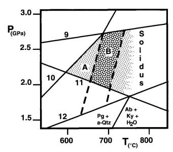
Fig. 7 P-T conditions defined for the high-pressure event (field A delimited by metamorphic reactions, the numbers correspond to the reaction numbers in the text). The two dashed lines, delimitning field B, correspond to the lower and higher temperature averages calculated for the Fe–Mg exchange between Cpx and Grt (samples collected in Unteralptal, Val Maighels and Val Nalps are considered).
