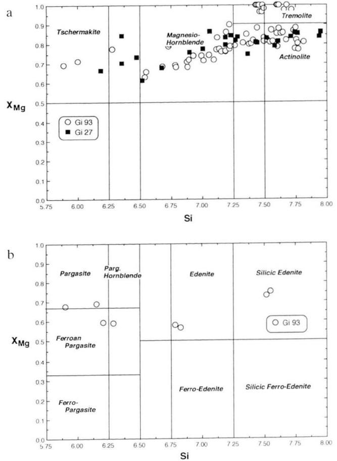
Fig. 8 Amphibole compositions from melagabbros. (a) for  $(\text{Na}+\text{K})_A < 0.5$ , (b) for  $(\text{Na}+\text{K})_A > 0.5$ . Amphibole nomenclature was calculated according to ROCK and LEAKE (1984).
