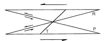
Fig. 8 Ideal fracture orientations in a sinistral strikeslip system. P and R are second order fractures and T is tension fracture. Notice that P and T fractures are oriented about 15° and 45° respectively off overall direction of shear. Modified from TIKOFF and TEYSSIER (1992).
