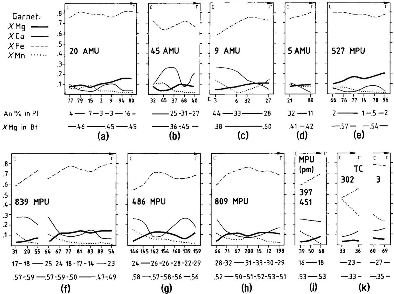
Fig. 6 (a–k) Synthetic garnet zonation profiles in XMg, XCa, XMn, XFe ( $X_n = n/(Mg + Ca + Mn + Fe)$ ), compiled and derived from core-rim (c, r) zonation profiles (Fig. 4). Small numbers refer to characteristic analyses in figures 2, 4, 5 of several porphyroblasts in each sample. Compositions of corresponding plagioclases and biotites (according to the microstructural criteria of Fig. 3) are expressed in An % and in XMg = Mg/(Mg + Fe) respectively.
