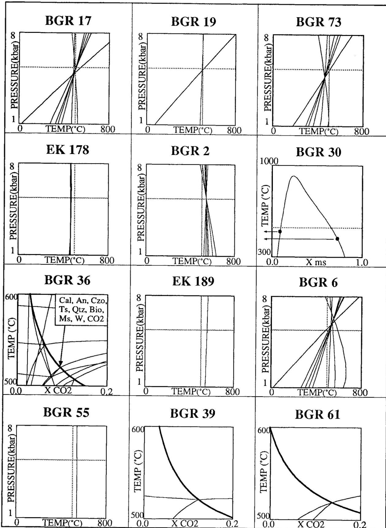
Fig. 7 Compilation of all the P-T, T-X<sub>CO<sub>2</sub></sub> and T-X ms equilibrium diagrams used to estimate metamorphic peak-conditions. Dotted crosses at 500 °C and 5 kbar plotted for reference. Information on chemical systems, reactants, reactions, fixed a<sub>H<sub>2</sub>O</sub> and fixed P respectively can be seen from table 2.
