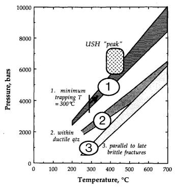
Fig. 6 Pressure-temperature diagram showing isochore ranges for fluid inclusion types 1, 2, and 3. Type 1 inclusions show bulk homogenization at ~300 °C, so must have been entrapped at higher temperature. Type 2 inclusions are on healed fractures that terminate at grain boundaries of ductilely deformed quartz. Type 3 inclusions are on late brittle fractures that crosscut all grain boundaries.
