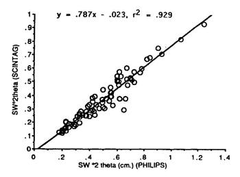
Figure 1 shows results of calibration measurements (85 samples) made on the PHILIPS 101 "analogue" diffractometer and on the SCINTAG XDS 2000 instrument. The samples were sedimented on glass plates  $(2.4 \times 4.8 \text{ cm})$  and air dried.
