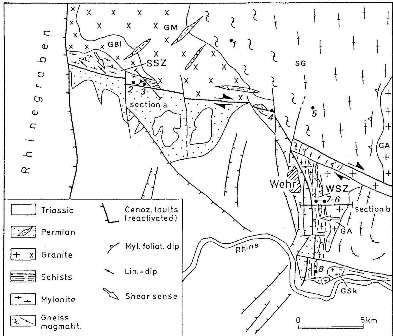
Fig. 6 Generalized geological sketch map of the southern Schwarzwald and stops. SSZ = Schlächtenhaus thrust zone; WSZ = Wehra normal shear zone. Variscan granites: GBI = Blauen granite; GM = Malsburg granite; GA = Albtal granite; GSk = Säckingen granite; see also table 1; SG = southern gneiss complex, in part migmatitic. Sections see figures 7 and 8 (after ECHTLER and CHAUVET, 1992).
