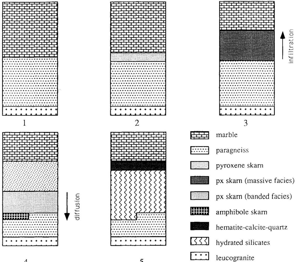
Fig. 3 Evolution of the skarn formation process in the main horizon: 1 = pre-metasomatic stage; 2 = metamorphic stage of the skarn; 3 = infiltration metasomatism during the prograde ore stage of the skarn (formation of the massive facies); 4 = diffusion metasomatism during the prograde ore stage of the skarn (formation of the banded facies); 5 = retrograde stage of the ore skarn. Abbreviation in the legend: px = pyroxene.
