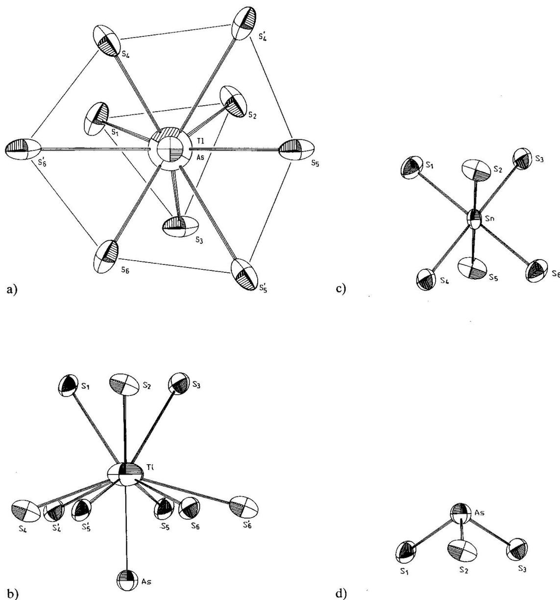
Fig. 6 Me-coordination polyhedra. a)  $TlS_6$ -polyhedron viewed along the  $c$ -axis; b)  $TlS_6$ -polyhedron rotated  $50^\circ$  around the  $a_2$ -axis; c)  $SnS_6$  trigonal antiprism; d)  $AsS_3$  trigonal pyramid.
