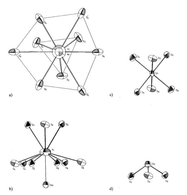
Fig. 6 Me-coordination polyhedra. a) TlS<sub>9</sub>-polyhedron viewed along the c-axis; b) TlS<sub>9</sub>-polyhedron rotated 50° around the a<sub>2</sub>-axis; c) SnS<sub>6</sub> trigonal antiprism; d) AsS<sub>3</sub> trigonal pyramid.
