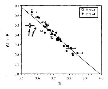
Fig. 6 Variation of (Al + F) and Ti in titanites from the pargasite (Br193) and the phlogopite (Br194) zones. The data are based on  $\Sigma$ (octahedrally coordinated cations) =  $\Sigma$ (Ti + Al + Fe<sub>tot</sub> + Cr) = 4.0. Error bars represent  $2\sigma$ -errors resulting from counting statistics. The plotted regression line has a slope of -1.405 ± 0.174, and a correlation coefficient of -0.934. Arrows point to outliers (see text for discussion).
