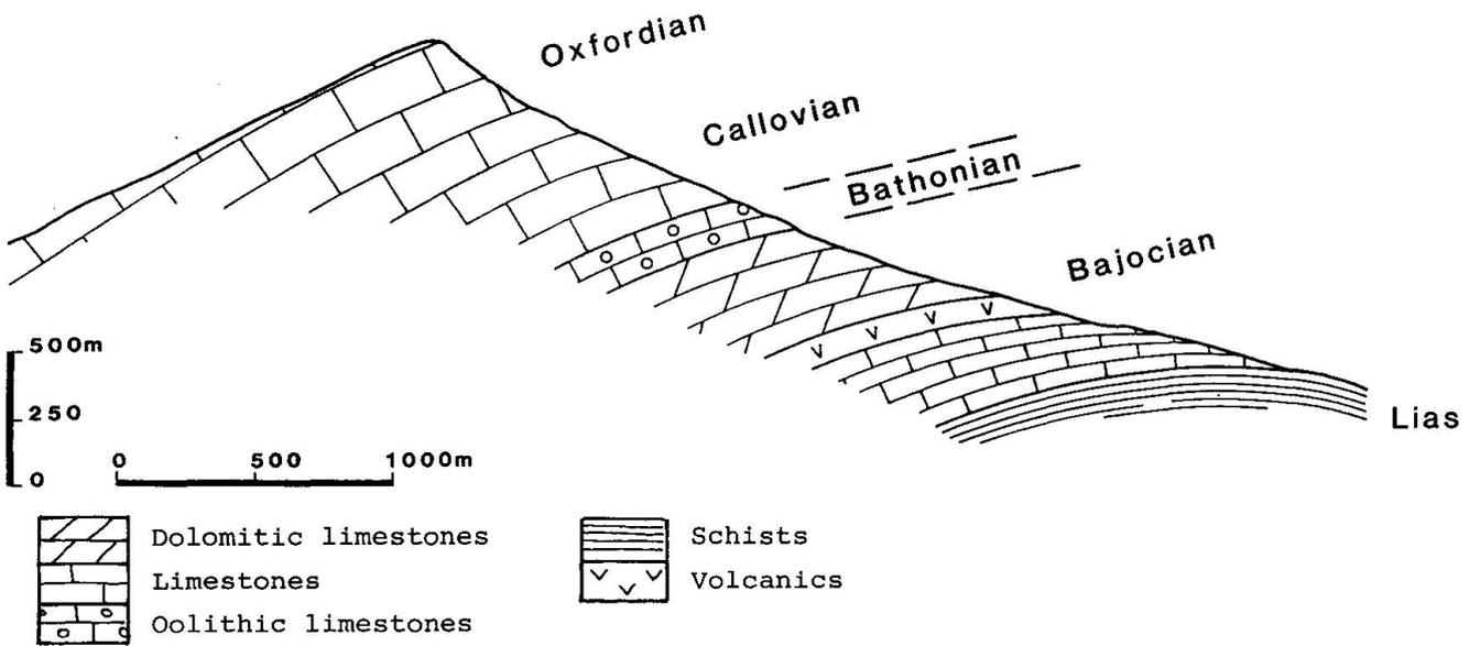
Fig. 2 Geological cross-section of Mount Hermon (Anti-Lebanon Range). Basalts underlie Bajocian limestones.
