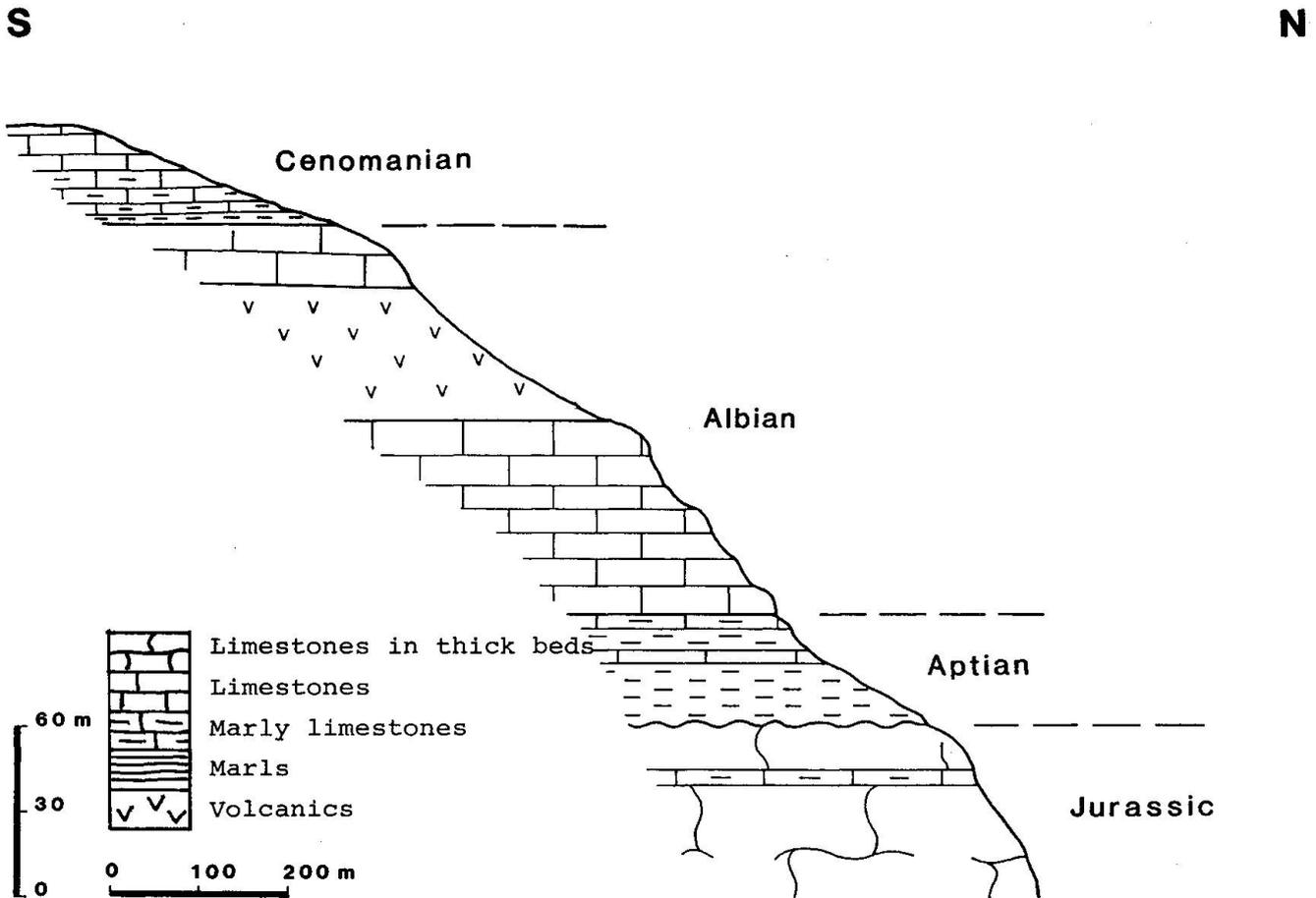
Fig. 4 Geological cross-section near Wadi Al Ouyoun (Coastal Range) showing the thick basaltic flow interbedded in the Albian sediments as seen on the western flank of the rift (Al Ghab).
