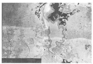
Fig. 7 SEM, BSE image, photomicrograph of sample 9: Penecontemporaneous braunite (br) and hollandite (hol) as principal manganese constituents, with pore-filling colloform hollandite and pyrolusite (pyr).
