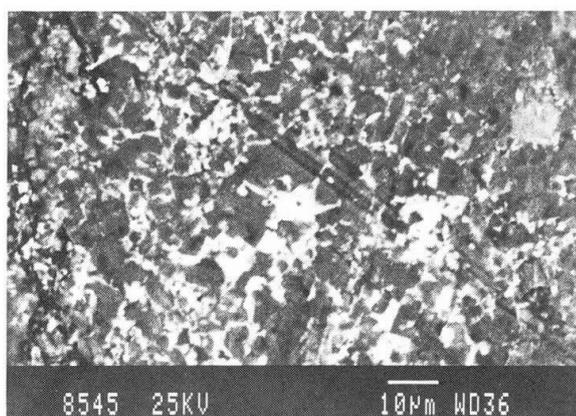
Fig. 9 SEM, BSE image, photomicrograph of sample 12: note hausmannite and coronadite intergrown in a mosaic texture.
