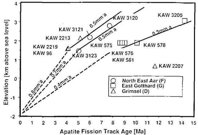
Fig. 6 Apatite age vs. elevation curves from the north-east Aar-, the eastern Gotthard- and the Grimsel region. The 1  $\sigma$  errors which are about 10% are given in table 1. KAW 96, KAW 575, KAW 576 and KAW 581 were taken from WAGNER et al. (1977).
