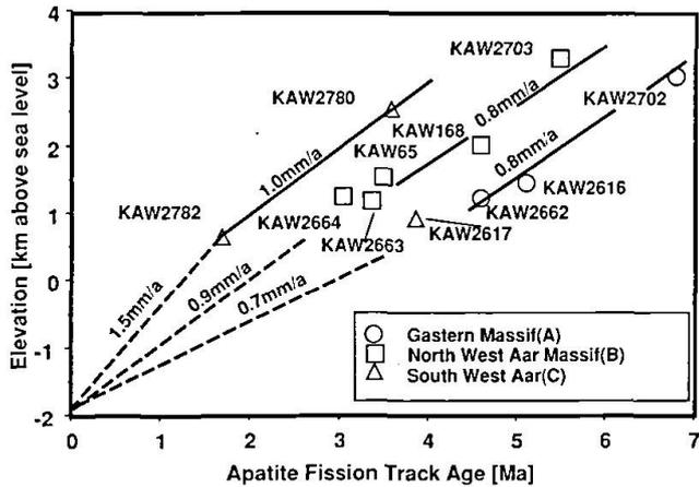
Fig. 5 Apatite ft age vs. elevation curves from the western part of the Aar massif. The 1  $\sigma$  errors which are about 10% are given in table 1. KAW 65 and KAW 168 were taken from WAGNER et al. (1977).
