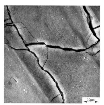
Figs 5 and 6 SEM pictures at higher magnification, showing the influence of beginning metamictization.
