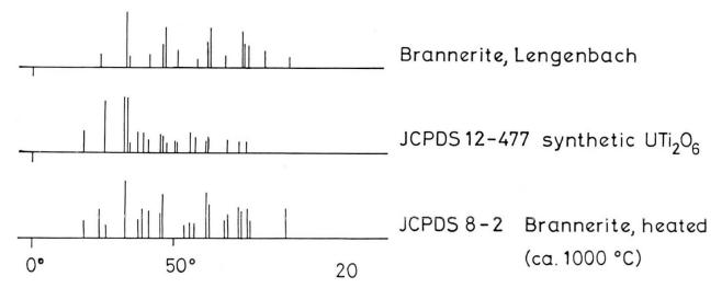
Fig. 2 Powder diagrams of brannerite: untreated, synthetic material, and natural brannerite (ignited at ca. 1000 °C).
