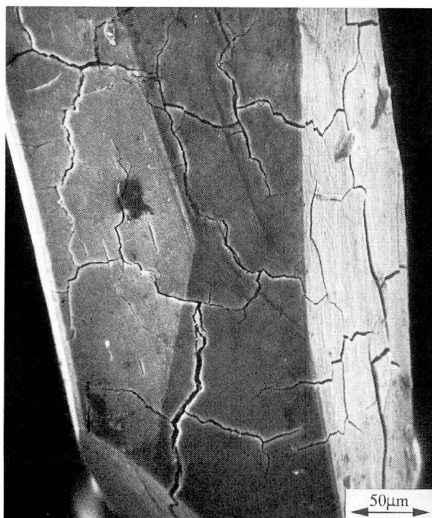
Figs 5 and 6 SEM pictures at higher magnification, showing the influence of beginning metamictization.
