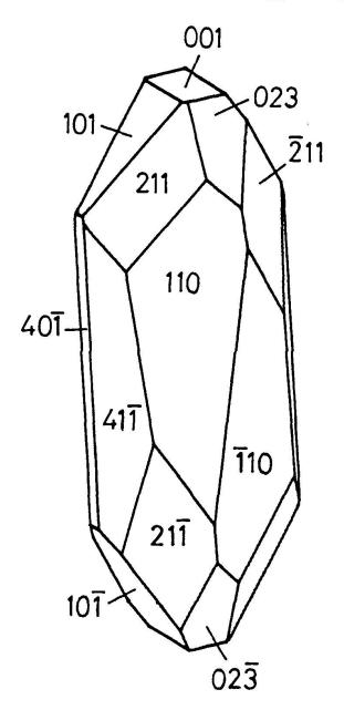
Fig. 4 Idealized crystal drawing according to the goniometrical measurement.
