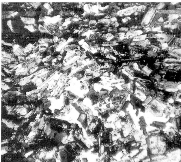
Fig. 13 Texture of microgranular enclave from the M. Capanne granite (Elba Island, Italy). The matrix has a fluidal texture deflected by a quartz oikocryst. Crossed polars. Diameter of quartz oikocryst: 2 mm. Crossed polars.
