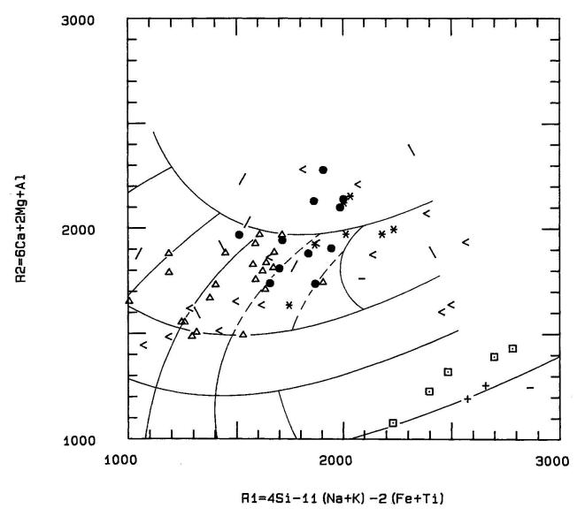
Fig. 3 R1-R2 classification (De La Roche et al., 1980). Symbols: Δ =NNW-amphibolites; ●=Mt. Vertana amphibolites; ★=Pennes metagabbro; ⊡=Fleres meta-andesites; +=Elzenbaum meta-andesites; /=Valtellina prasinites; \= Camonica valley amphibolites; < = Val di Sole amphibolites.
