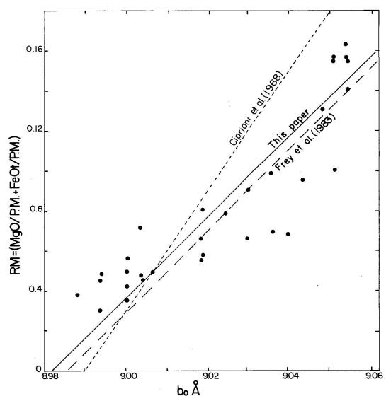
Fig. 4 Correlation of b<sub>0</sub> and R.M. Dotted and broken lines represent the equation of CIPRIANI et al. (1968), FREY et al. (1983) respectively. The best fit line to 32 data of Verrucano muscovite is also shown.
