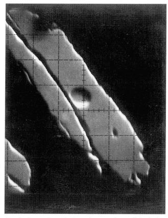
Fig. 1 Secondary electron image of a polished zircon formed co-magmatically at ca. 870 Ma in the gabbroic protolith of a retrograded eclogite of the Gotthard Massif. The 20–30 μm big and 2–3 μm deep crater was produced by oxygen-induced sputtering using SHRIMP. For cathode-luminescence distribution of this grain see Fig. 3.
