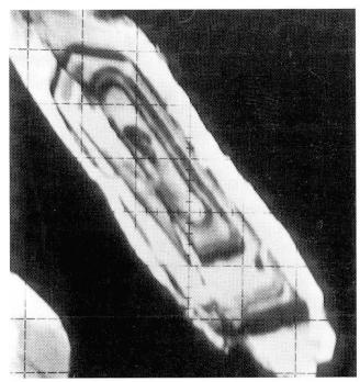
Fig. 3 Cathode-luminescence image of the grain shown in Fig. 1 (width ca. 60 μm). Multiple euhedral zoning is indicated by the different C.L. response which is largely based on variable sums of trace and minor elements. Probably, this grain grew under variable P-T-X conditions during formation and ascent of the gabbroic protolith.
