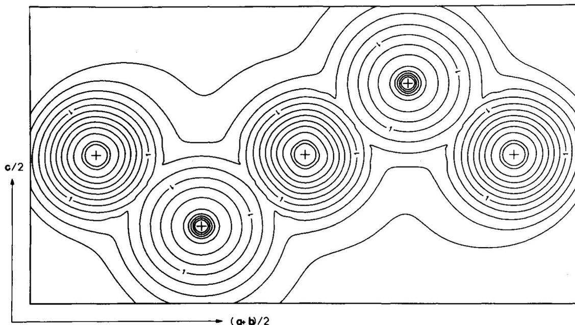
Fig. 2 Electronic charge density distribution in  $e/\text{\AA}^3$  in the plane (110), total density; successive contour lines differ by a factor of 2. The position in the center of the Figure refers to Cu.
