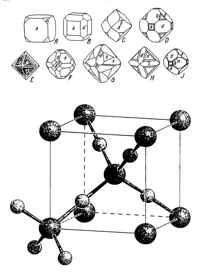
Fig. 1 Projection of the crystal structure of cuprite, Cu<sub>2</sub>O. Large spheres: oxygen; small spheres: copper. The morphological drawings A-J on top are from Niggli (1926); a-x indicate the different face forms (cf. p. 218).
