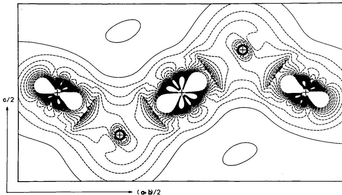
Fig. 3 Difference between the density computed for a nine-atom cluster and the density computed for the  $\text{Cu}^+$ ,  $\text{O}^{2-}$  ions in the plane (110). Negative contours are broken; increment is  $0.05 e/\text{\AA}^3$ . Note the reduced electron density in  $\text{Cu}^+$ : net positive charge about  $0.45 e$ , and enhanced density in  $\text{O}^{2-}$  ions: net negative charge about  $0.90 e$ .
