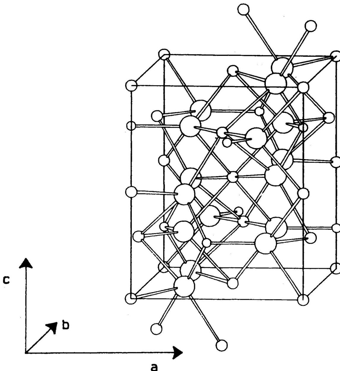
Fig. 5 Projection of the crystal structure of forsterite,  $Mg_2SiO_4$ . Large circles: oxygen at two positions 4c (point symmetry  $m$ ) and one position 8d (point symmetry 1); medium circles: magnesium at positions 4a (point symmetry 1); small circles: silicon at position 4c of space group  $Pbnm$ .
