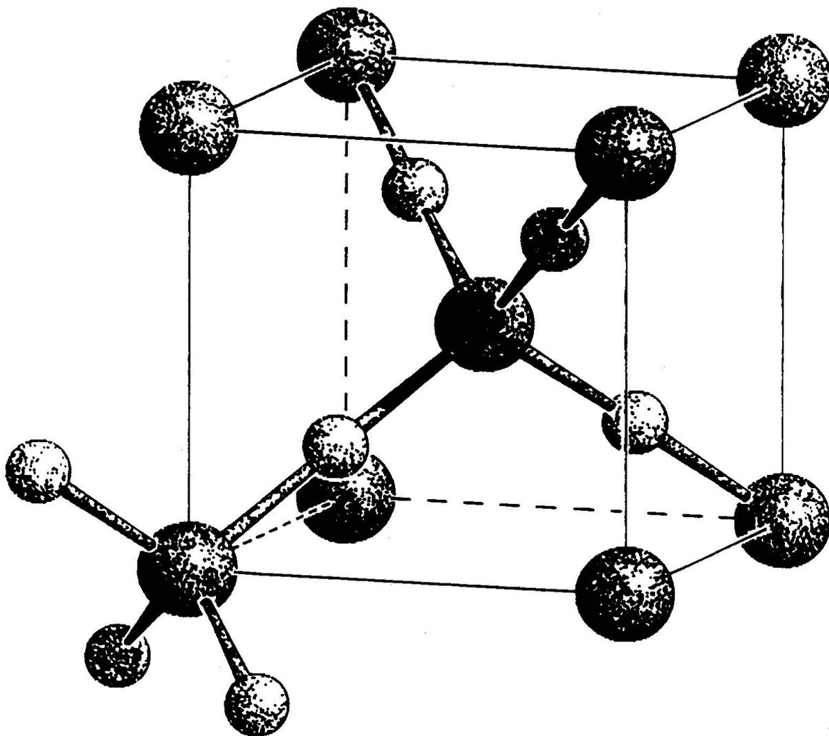
Fig. 1 Projection of the crystal structure of cuprite,  $\text{Cu}_2\text{O}$ . Large spheres: oxygen; small spheres: copper. The morphological drawings A-J on top are from NIGGLI (1926); a-x indicate the different face forms (cf. p. 218).
