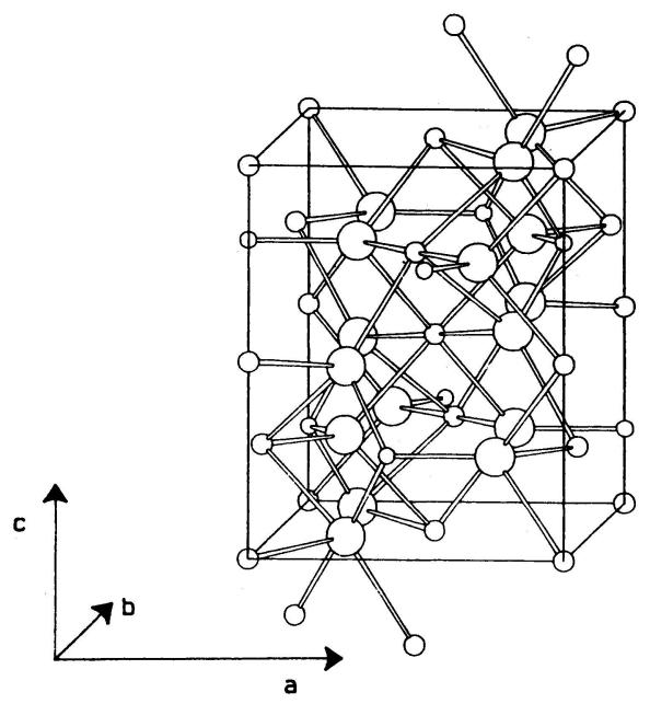
Fig. 5 Projection of the crystal structure of forsterite, Mg<sub>2</sub>SiO<sub>4</sub>. Large circles: oxygen at two positions 4c (point symmetry m) and one position 8d (point symmetry 1); medium circles: magnesium at positions 4a (point symmetry 1); small circles: silicon at position 4c of space group Pbnm.
