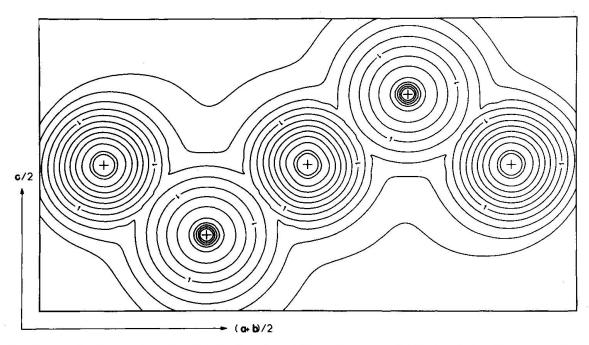
Fig. 2 Electronic charge density distribution in  $e/A^3$  in the plane (110), total density; successive contour lines differ by a factor of 2. The position in the center of the Figure refers to Cu.
