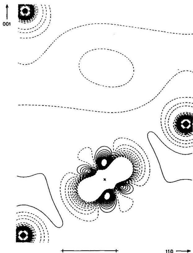
Fig. 4 Static model deformation map of RESTORI and SCHWARZENBACH (1986, Fig. 2(d)), in the plane (110) as in Fig 3. Contours drawn between  $\pm e/A^3$ , negative contours broken. The map is comparable to the one of Fig. 3.
