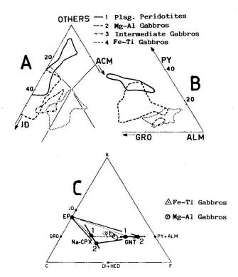
Fig. 2. Relationships between mineral chemistry and primary lithology compositions: Na-clinopyroxenes (A) and garnets (B). (C): ACF-type projection (from QZ, H<sub>2</sub>O, CaAlNa<sub>-1</sub>Si<sub>-1</sub>, FeAl<sub>-1</sub>, MgFe<sub>-1</sub>; Thompson, 1981) showing chemographic relations for the eclogitic Mg-Al-gabbros and Fe-Ti-gabbros (Messiga, 1987).
