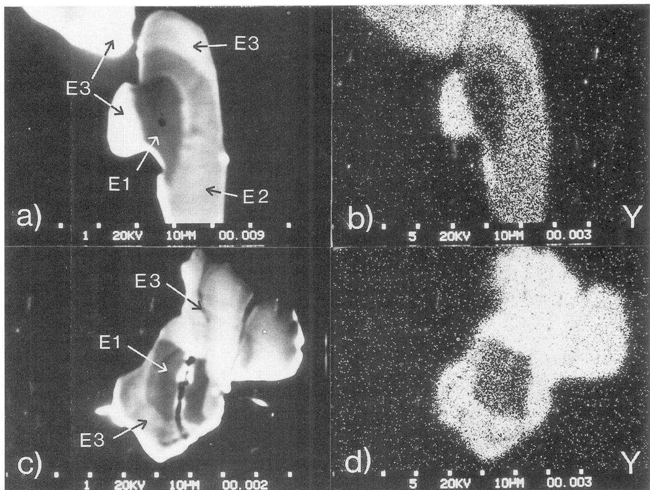
Fig. 1 a) Secondary electron image of zirconolite showing three zones E1, E2 and E3. b) X-ray distribution of Y. c) Secondary electron image of zirconolite displaying two zones E1 and E3. d) X-ray distribution of Y. Microprobe analytical conditions were 20kV and 25nA measured on a Faraday cage.
