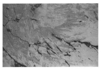
Fig. 3 Section of Fig. 2 but viewed under oil immersion. Oriented unidentified exsolutions with slightly lower reflectance become visible within the cervandonite-(Ce) matrix (maximum dimension of the photograph is approximately 100 μm).
