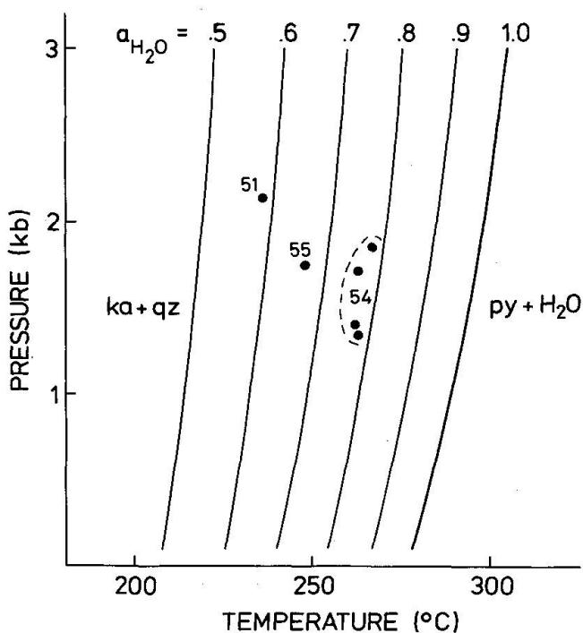
Fig. 3 Calculated P-T stability limits for the reaction  $\text{kaolinite} + \text{quartz} = \text{pyrophyllite} + \text{H}_2\text{O}$  at different water activities. The P-T conditions from Table 1 for localities 51, 54 and 55 at the reaction-isograd are indicated.
