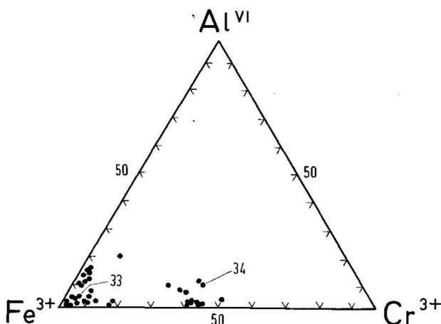
Fig. 9 Aegirine and chromiferous aegirine-augite in emerald-green quartzite. The Cr contents define a compositional gap between aegirine ( $Fe_{tot} = Fe^{3+}$ ) and aegirine-augite ( $Fe_{tot} = Fe^{3+} + Fe^{2+}$ ). The numbered dots refer to analyses listed in table 4. The analyses are from 4 samples.
