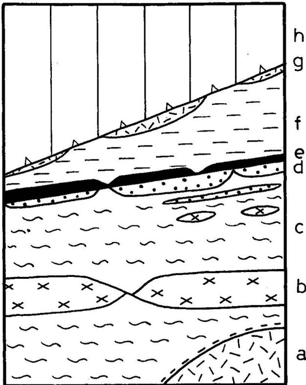
Fig. 3 Sketch of the lithologic sequence in the St. Marcel valley. a) serpentinized peridotite tectonites; b) metagabbro bodies; c) garnet-rich glaucophanitic metabasalts; d) chlorite-schists and prasinites; e) manganiferous quartzites; f) calcschists, marbles and associated micaschists; g) serpentinite mylonites; h) Austroalpine Mt. Emilius Klippe.
