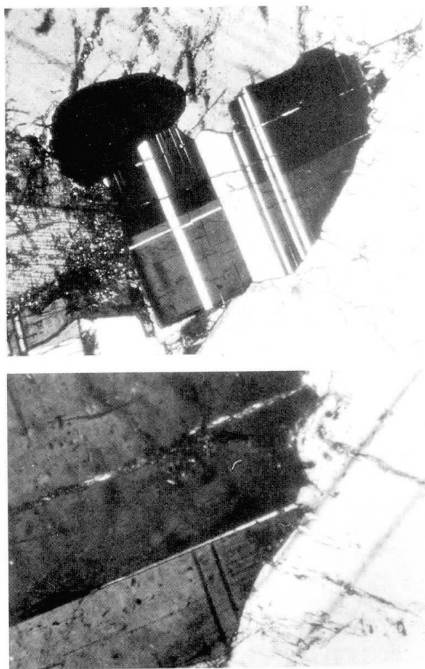
Fig. 3 Microphotograph of a typical simple Ala-A twin with transverse albite-law lamellae cutting straight through the composition plane (CP). Note the almost equal extinction positions of the Ala individuals: in a section exactly normal to [100] the twin would be invisible. A thin acline lamella very close to the Ala CP (right, enlarged in (b)), and a somewhat broader pericline lamella (left, some distance above this CP) both form a "pseudo-Manebach law" with the opposite Ala individual. Crossed polars. Width of photograph (a) 1.5 mm.
