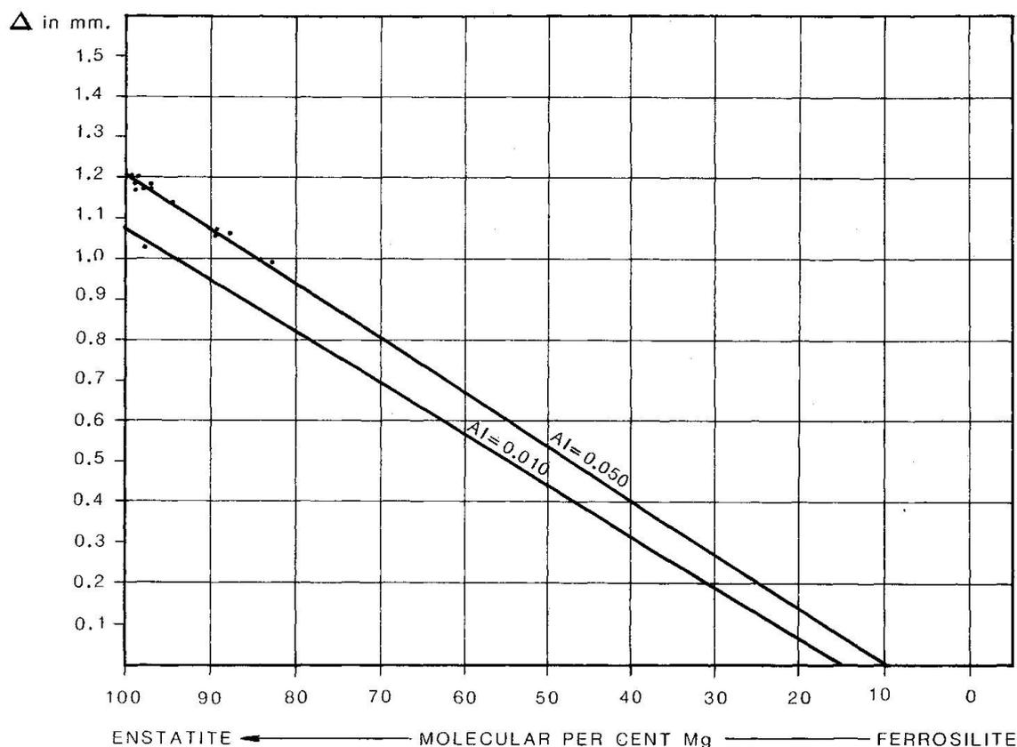
Fig. 5  $\Delta$  is the relative distance in millimeters between X-ray reflections 10 3 1 and 060 for a range of orthopyroxenes (after ZWAAN, 1955). The dots refer to measurements on X-ray powder photographs, exclusively taken, using Fe-radiation and a camera with a diameter of 114.6 mm.
