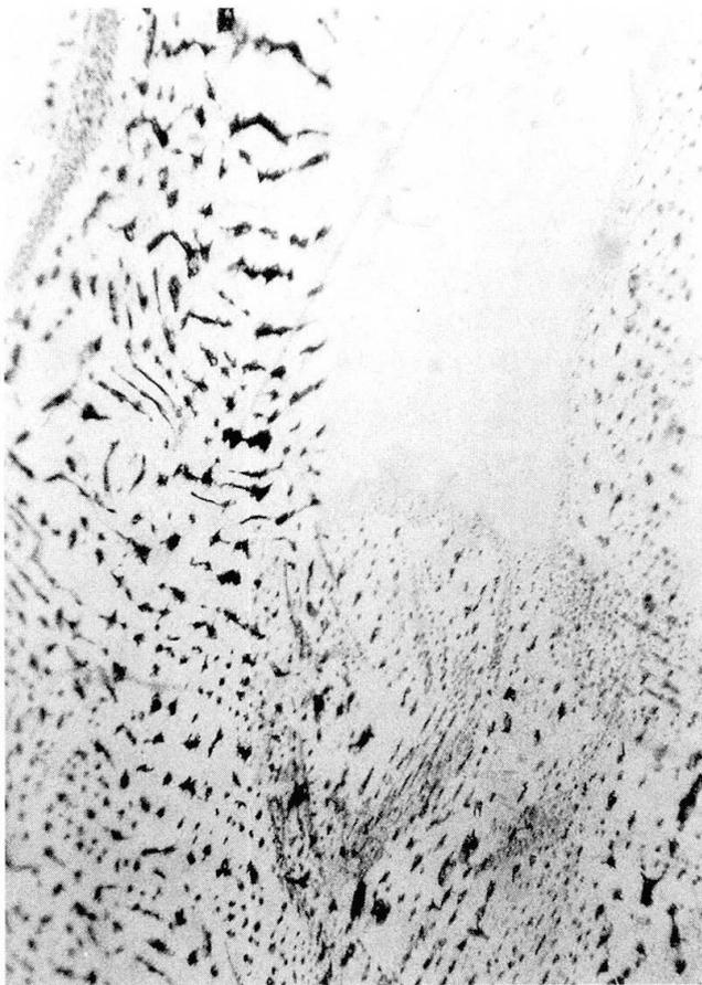
Fig. 4 Liquid feathers and two-phase inclusions in colourless enstatite RGM 152034 ( $\times 15$ ).
