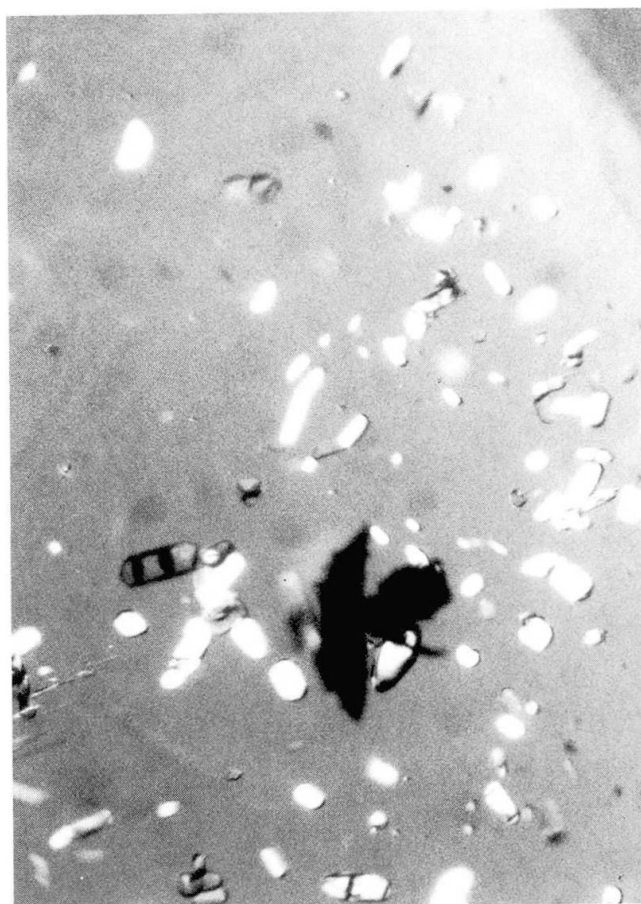
Fig. 3 Quartz crystals included in colourless enstatite RGM 152003 ( \times 30 ), polarized light.
