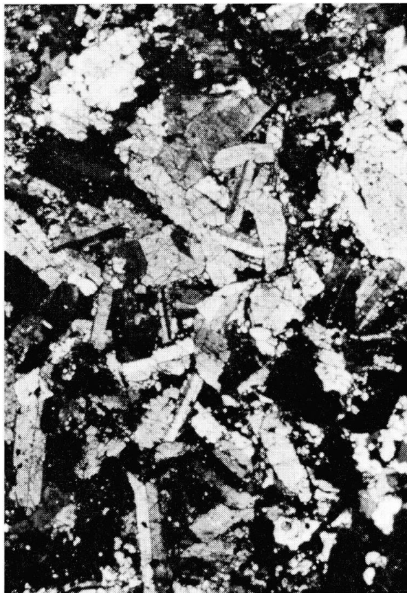
Photograph 2 (width: 3.3 mm). Andesitic rock component with albite laths.
