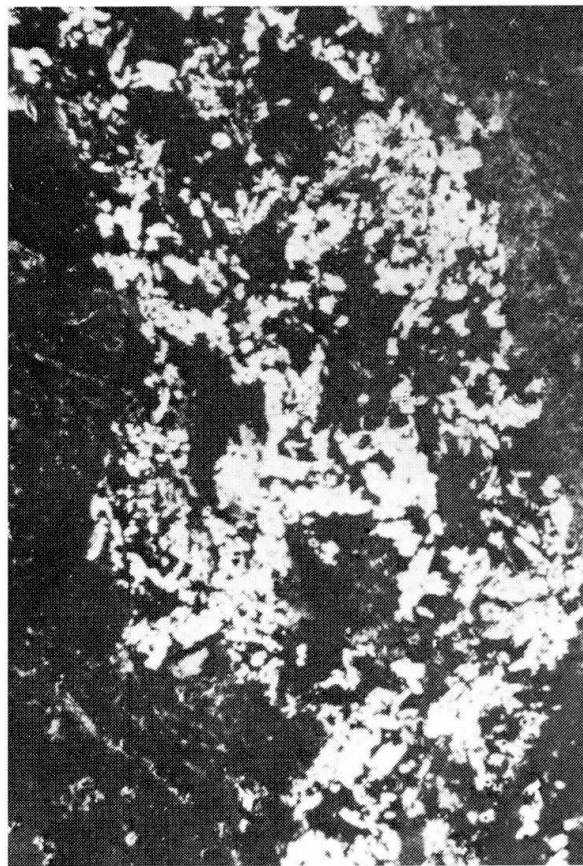
Photograph 3 (width: 1.0 mm). Brannerite (light band in upper part of photograph) and pitchblende in a fine network. Area of photograph 4 is marked as a white square.
