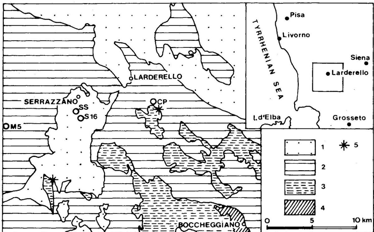
Fig. 2 Geological sketch map of the Larderello region and location of the studied wells. 1. Neogene sediments. 2. Ligurids. 3. Tuscan Nappe. 4. Boccheggiano Formation s.l. 5. Small outcrops of Verrucano. Open circles: studied wells. For symbols see text.
