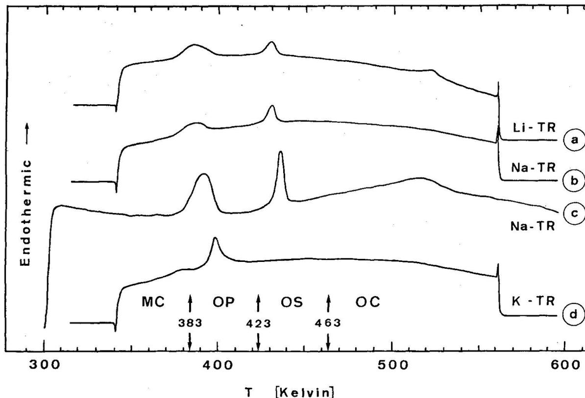
Figure 4 Tracings of the DSC scans for synthetic alkali- $\text{WO}_4$  fluxgrown tridymites over narrow temperature ranges. Scans a, b and d are first heating-scans from 340 to 560 K on the lithium, sodium and potassium fluxed preparations. Same instrument settings as in Figure 1 were used. The sample weights were about 24 mg for Li-TR and 30 mg for Na-TR and K-TR respectively. Scan c was made from 300 to 600 K on the DSC-2C, and revealed the 517 K peak in Na-TR.
